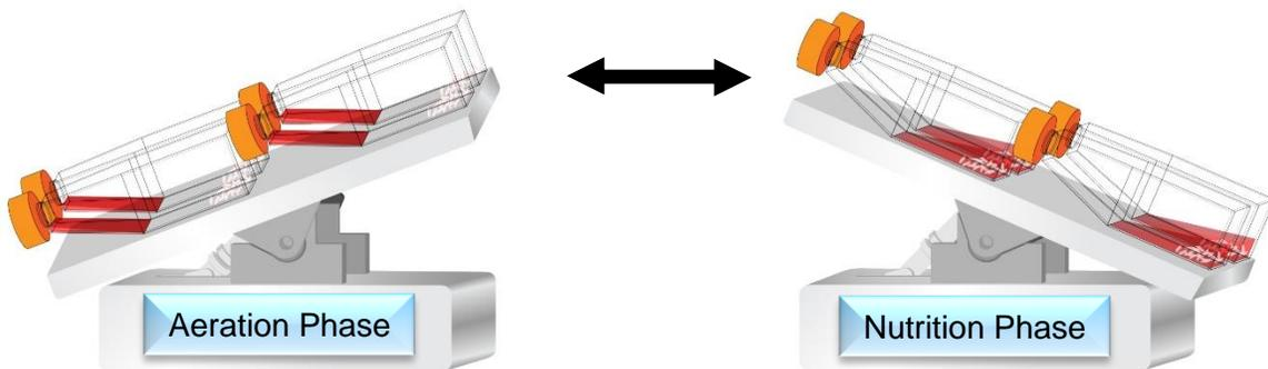
**Figure 2:** The Mini Tide Motion System serves as a small-scale system to conduct initial process optimization. The carriers are seeded with cells and aseptically transferred into tissue culture flasks positioned on a rocker (Figure 2); this setup simulates the Tide Motion observed in CelCradle™.
