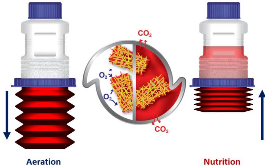
**Figure 1:** CelCradle™ operates via Tide Motion with adherent cells attached to BioNOC™ II carriers. The packed bed is exposed to aeration and nutrition phases via decompression and compression of bellows.
